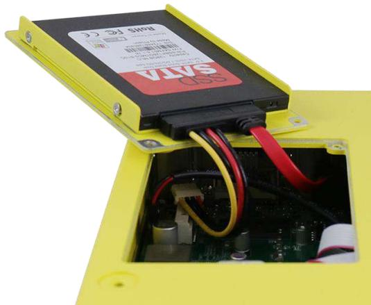
5. Gently put the tray back into the system with the connector side being inserted into the system first and secure the tray with three screws.
