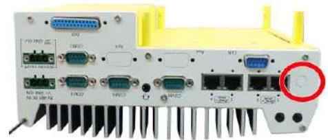
For Nuvo-9100/ 9200VTC systems, the ignition control rotary switch can be found on the MezIO™ once you disassemble the enclosure.
