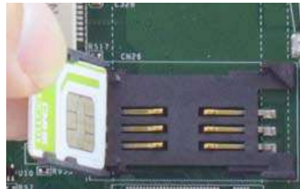
Insert Mini-SIM card with pins facing up
