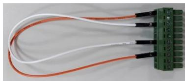
Rx of ttyS1 and Tx of ttyS2 are connected (orange wire), while Tx of ttyS1 and Rx of ttyS2 are connected (white wire). With this wiring, messages from ttyS1 is sent to ttyS2 over RS-232, while message from ttyS2 is sent to ttyS1.
